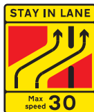
One lane crossover at contraflow road works
