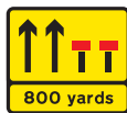
Temporary lane closure (the number and position of arrows and red bars may be varied according to lanes open and closed)
